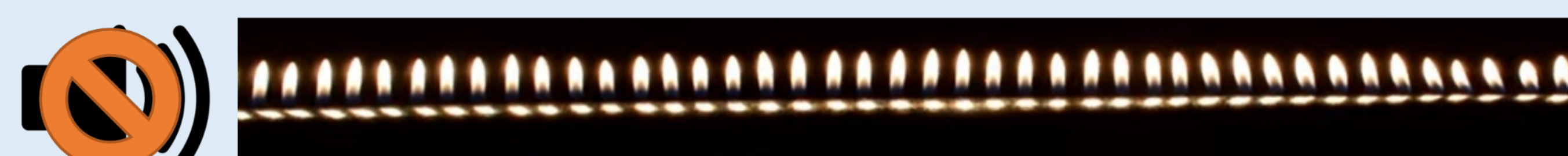
Uniform molecular density | Uniform pressure Uniform flame heights
